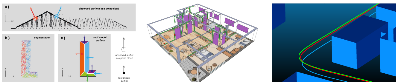
Figure 1: Three examples for AI applied in geoinformation, left: Classification and reconstruction of roof models from 3D point clouds. Middle: Reasoning for automatic estimation and detection of invisible electrical wires in the wall. Right: Improving vehicle trajectories using 3D city models.
