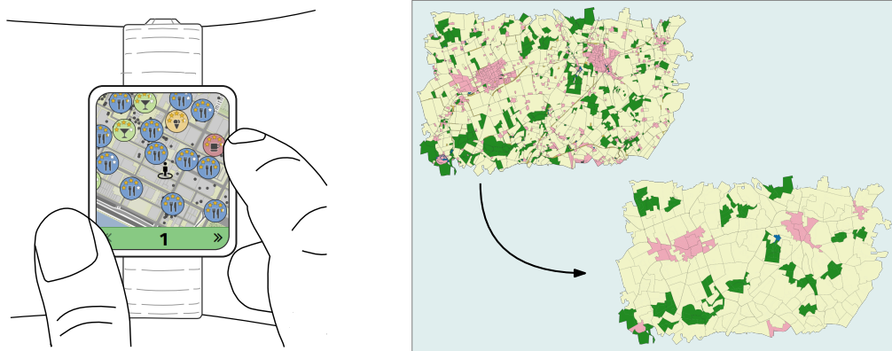
Figure 1: Two application examples for automation in cartography. Left: Map with labeled POIs on a smartwatch. Right: Generalization of a topographic map.
